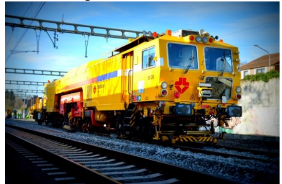
Figure 6.3 Leonardo inspection vehicle (Strukton Rail NV)
